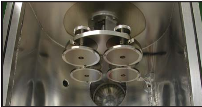
This custom flat planetary features instantly removable carriers for convenient, benchtop substrate mounting or cleaning. This assembly accommodates (4) 4" wafers or numerous smaller substrates. Larger versions up to (4) 300 mm wafers are also available.
