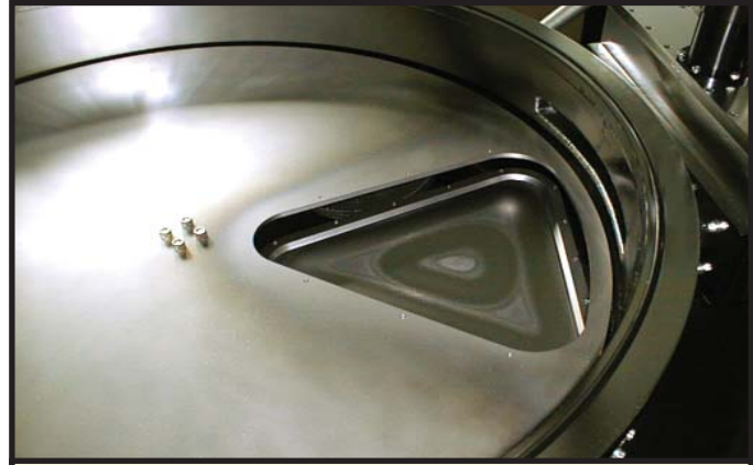
The AJA TR5313 triangular magnetrons are specialty sources designed to optimize deposition uniformly onto a circle of substrates up to 8" diameter.
