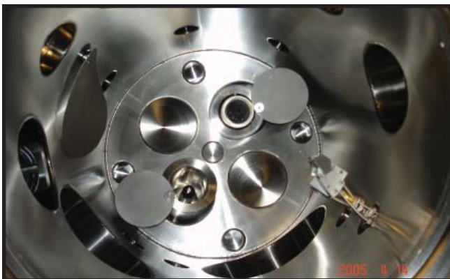
40 cc KNUDSEN CELL and Ti BALL EVAPORATOR in W/C CHIMNEYS
