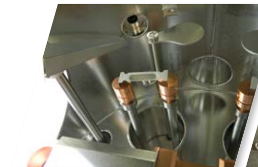
Secondary Thermal Evaporation Source with In-situ Refill Mechanism
