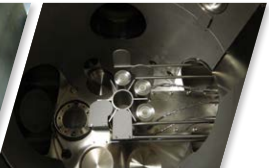
Up to 6 thermal evaporation furnaces on easy access slide rail
