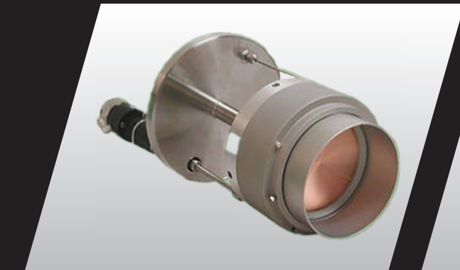
A340-XP Source 4" Target UHV magnetron sputtering source on 8" CF rotatable flange (bolt ring not shown) with chimney, gas ring and pneumatic shutter.
