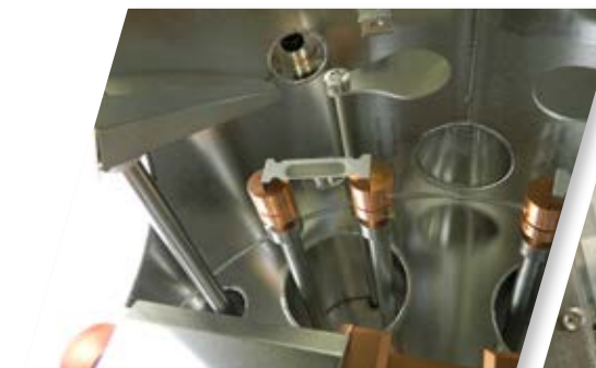
Secondary Thermal Evaporation Source with In-situ Refill Mechanism
