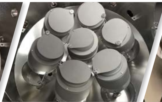
(6) 3” UHV magnetron sputtering sources in confocal arrangement, (1) 3” sputter source in direct deposition orientation
