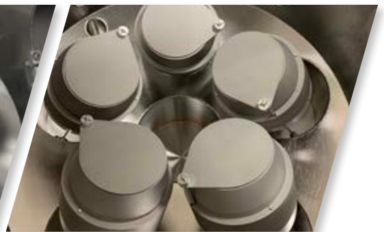
(5) 4” UHV magnetron sputtering sources in confocal arrangement
