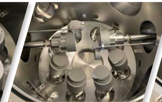
Accommodates up to (13) sputtering sources with confocal, direct and off-axis orientation
