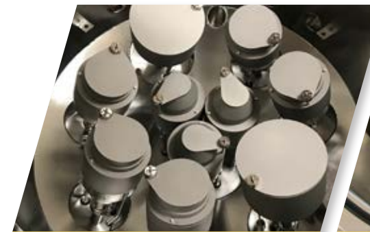
(8) 2” UHV magnetron sputtering sources in confocal geometry, (2) custom anti-shorting sputtering sources optimized for chalcogenide materials
