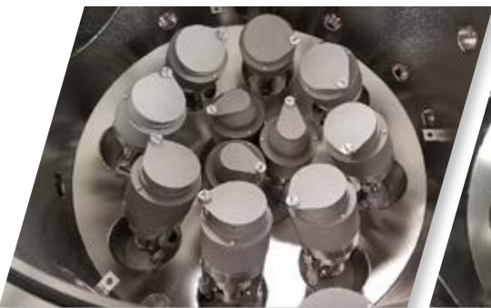
(11) 2” UHV magnetron sputtering sources in confocal arrangement
